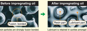
Resin particles are strongly fusion bonded.
