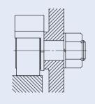
Fig. 7 Mounting of C-Lube Unit
