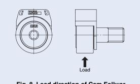
Fig. 8 Load direction of Cam Follwer
